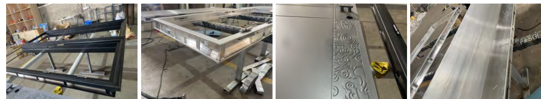
SECURITY DOOR LOCK 8MM ALUMINUM PANEL ALUMINUM HONEYCOMB PANEL 8MM ALUMINUM PANEL DOOR CASE
